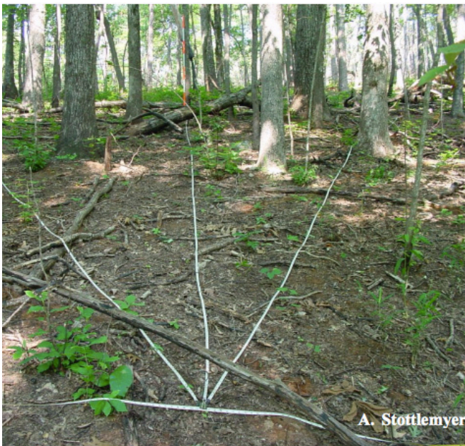
Image 7.11. Example of transect lines used with the planar intercept method to assess fuel loads, horizontal fuel continuity, litter depth and duff depth. Image courtesy of Aaron Stottlemeyer.
