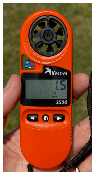
Image 3.10. Kestrel Weather Meter. Image courtesy of Leslie Boby.
